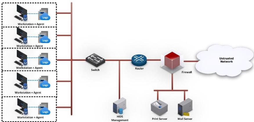
Figure 2: A typical network topology of a HIDS
