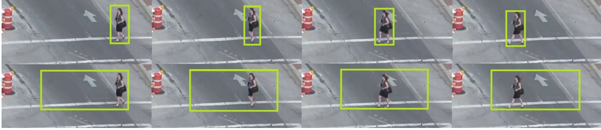
Figure 1: First row: frames sequence with the detected object by YOLOv4 [26]. Second row: frames sequence after EABBox creation.
