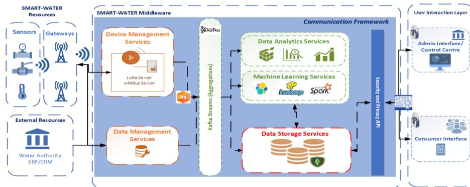
Fig. 2. Basic components of SMART-WATER system architecture
