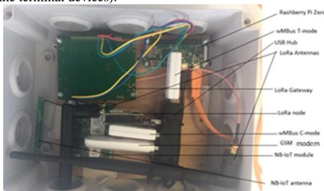
**Fig. 1.** Custom gateway and its electronic components
