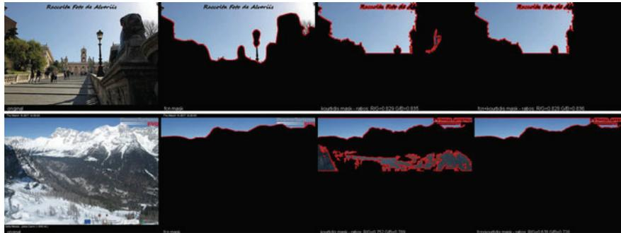
**Fig. 5.5** Comparison of the masks generated by the *FCN* approach (2nd column) with the masks generated by the *heuristic* approach (3rd column) for the images of the 1st column. The 4th column shows the masks generated by the *FCN+heuristic* approach
