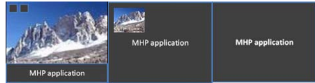
Figure 10 Card Display Modalities: Stripe, Full Screen with TV Picture, and Full Screen Instance of a Multimedia Page
